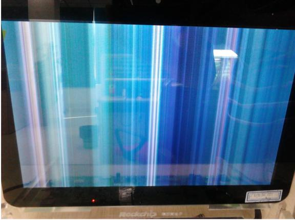
As shown picture below, we call it "Ghosting", there is a similar situation triggered by the incompleted reference layer of the board. The way to fix it is trying raise the VCC\_DDR voltage to 1.6V or bypassing the dll of DDR.
