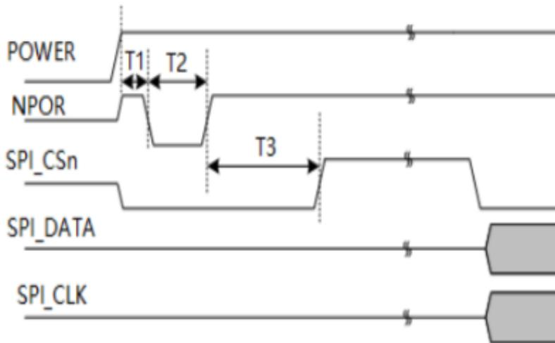
$T1 > 0, T2 \geq 1ms, T3 \geq 3ms$
