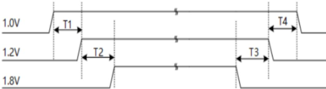
$T1 \geq 0, T2 \geq 0, T3 \geq 0, T4 \geq 0$
