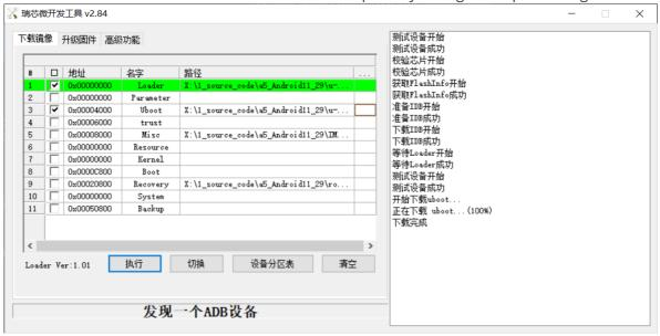
You can use FactoryTool to flash update.img compiled and generated in step5 during mass production.
