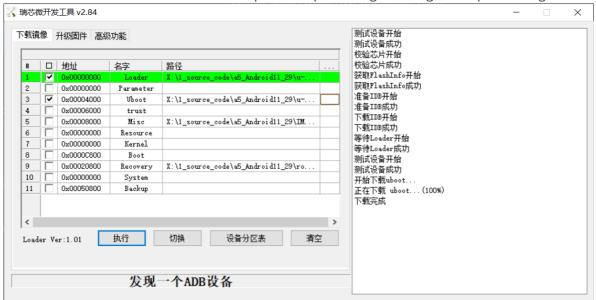
You can use FactoryTool to flash update.img compiled and generated in step4 during mass production.
