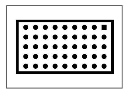
The test will find the circle closest to the center, so exact alignment is not required. As the test zooms, some of the circles will be cropped out of the image. Provided a full circle can be found in the image, the test can run at the zoom level selected.
