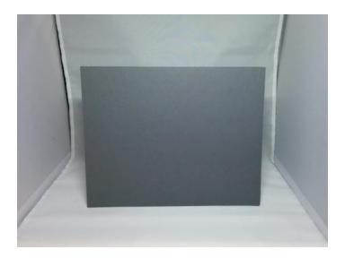
In particular, the grey card must be roughly centered in the field of view, taking up around  $\frac{1}{2}$  x  $\frac{1}{2}$  of the scene, with the white background visible on all sides around it. As is evident from the image above, a high degree of precision is not required; the most important factors are that the scene is completely static (including no light source flicker) and that the very center of the image is within the grey card area.
