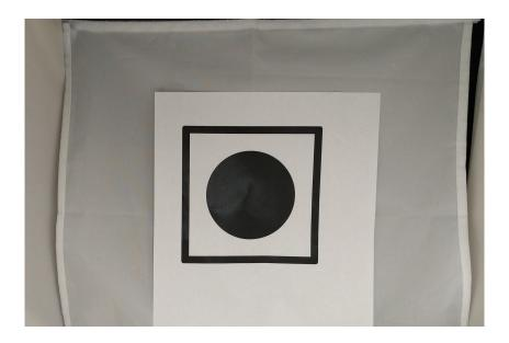
Make sure the square box is completely included in the picture, and no other complicated background is exposed in the scene except the original white one. Place the camera right in front of the test page, so that each of the four edges of the square is roughly parallel to its corresponding border of the picture. Do not point the lighting source directly at the test chart, or allow the black circle to be over-exposed.
